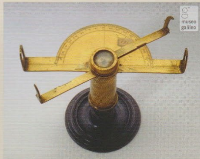
Graphometer, an early 17th-century land surveying instrument
